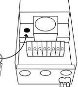
Your Transformer is provided with a long loop in the optional photocell plug that you may utilize to measure the input current. Simply apply the clamp on the Amp Meter around the loop and measure the current. (See Chart 3)
